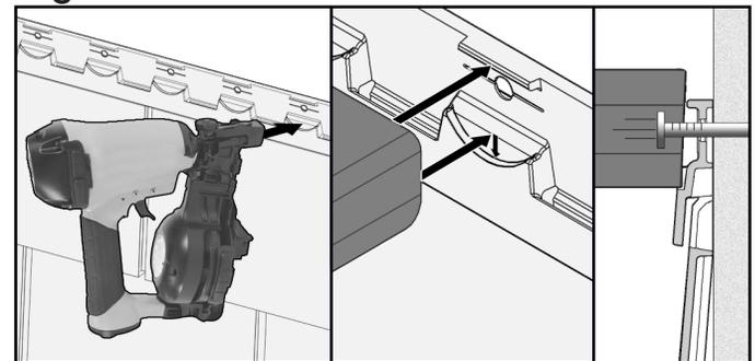
4-Make sure that all pieces are properly joined together (push firmly upwards on the section making sure that the insertion is complete) (Figure 4).
