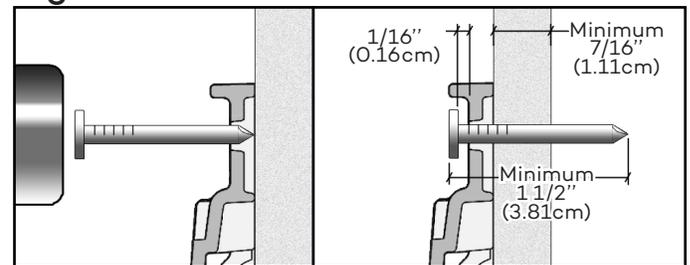
3-The Beach House Shake nailing channel allows the use of roofing nailer (ex: Bostitch RN46 and Hitachi NV45). To do so, adjust the tip of the nailer at the highest position. Push the nozzle into the cavity under the nail holes and push against the product to nail. Make sure each nail is aligned in the nailing hole. (Figure 3)
